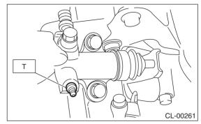
7) After depressing the clutch pedal, make sure that there are no leaks evident in the entire system.8) After bleeding air from system, ensure that the clutch operates properly.
