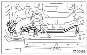
7) Disconnect the ATF cooler hoses from the pipes. NOTE:
