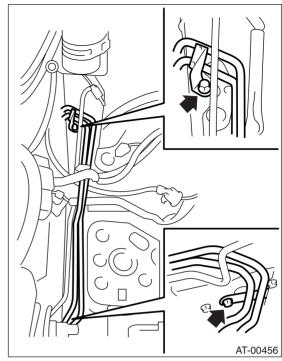
9) Remove the ATF cooler inlet and outlet pipes.
