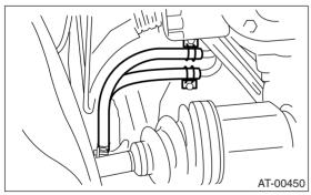
8) Disconnect the ATF cooler pipe from frame.
