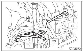
2) Install the ATF cooler pipe to frame.
