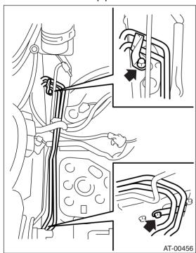
3) Connect the ATF cooler hose to the pipe on the transmission side.
