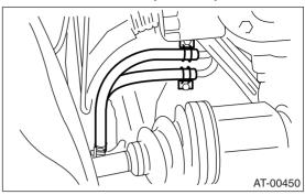
4) Connect the ATF cooler hose to the pipe on the radiator side. (Non-turbo model)
