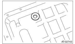
4) Apply proper amount of liquid gasket to the entire oil pan mating surface.
