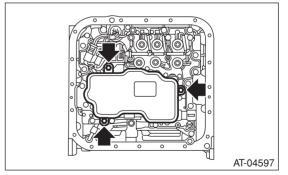
3) Attach the magnet at the specified position of the oil pan.
