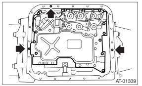
6) Install the oil pan by equally tightening the bolts.
