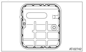
5) Fill the three holes aside from the bolt holes in the transmission case, with liquid gasket.
