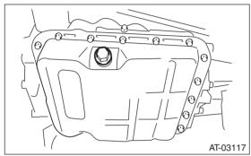
6) Perform replacement with a new gasket, and tighten the drain plug (ATF).
