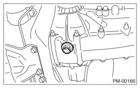
2) Replace the gasket with new one, and then tighten the drain plug to specified torque.
