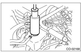
2) Check the radiator cap valve open pressure using radiator cap tester.
