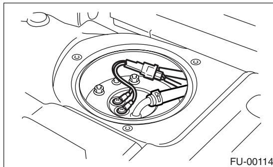
8) Remove the bolts which install fuel sub level sensor on fuel tank.
