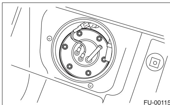
9) Remove the fuel sub level sensor.
