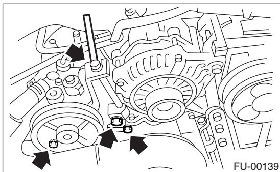
(4) Install the power steering pipes onto the fuel pipe protector RH.
