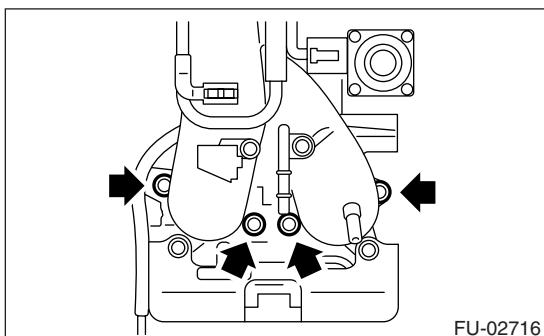
20) Remove the intake manifold.
