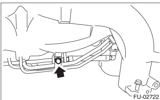
20) Remove the fuel pipe from intake manifold.
