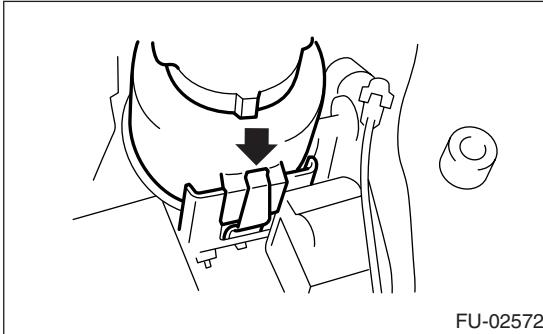
(2) Connect the power steering pump switch to the connector (A).
