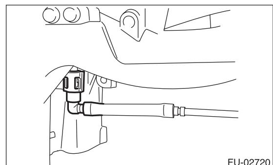
4) Install the fuel injector.
