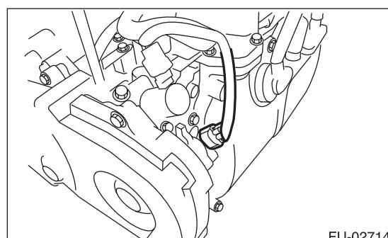
5) Connect the connector to the power steering pump switch.
