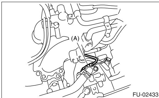
(3) Install the installation bolt of the power steering pump bracket.
