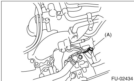
7) Connect the connector to crankshaft position sensor.
