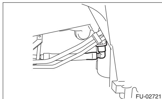
3) Connect the fuel injector pipe RH to the fuel pipe.
