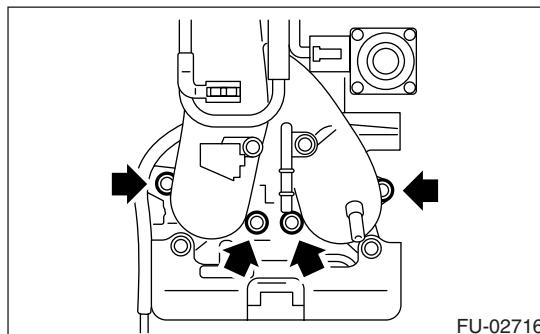
2) Connect the fuel hose and evaporation hose to the fuel pipe.
