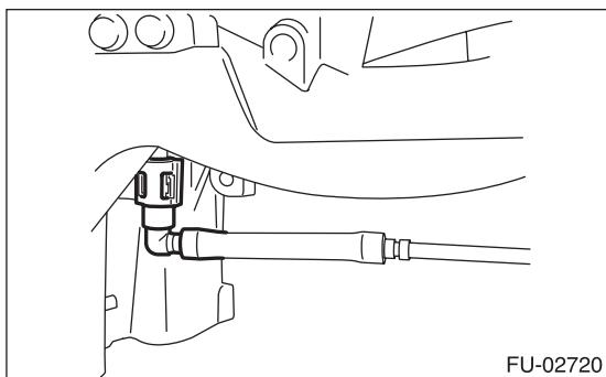
17) Disconnect the quick connector that fastens the fuel injector pipe LH to the fuel pipe.
