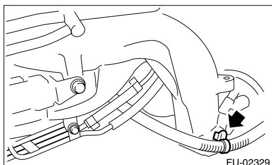
12) Remove the bolts which hold engine harness to intake manifold.
