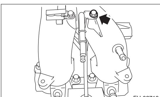
15) Remove the fuel injectors from injector pipe.
