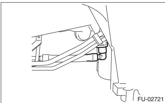
18) Remove the fuel injector pipe RH and LH.
