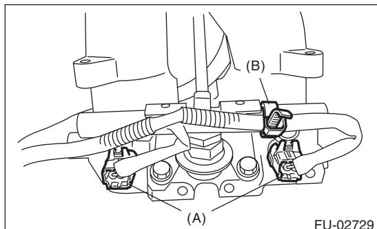
10) Remove the purge control solenoid valve.
