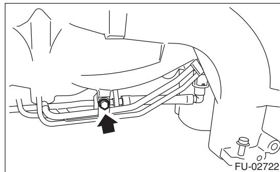
2) Connect the fuel injector pipe LH to the fuel pipe.
