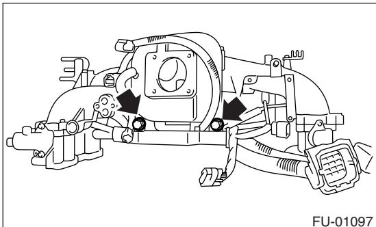
13) Remove the engine harness from intake manifold.
