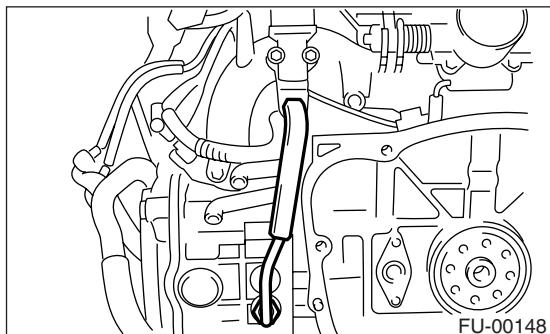
18) Disconnect the fuel hoses from fuel pipe.
