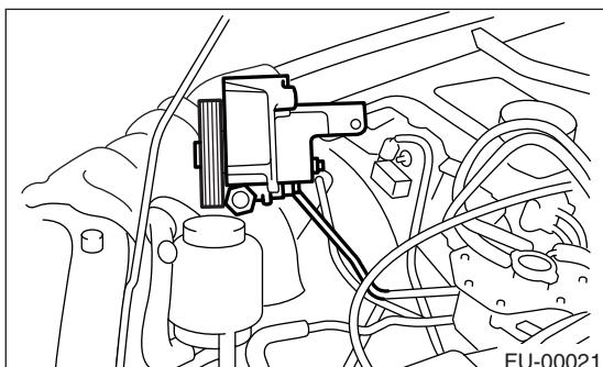
7) Remove the spark plug cords from the spark plugs by pulling the plug caps. (Do not pull the cord.)
