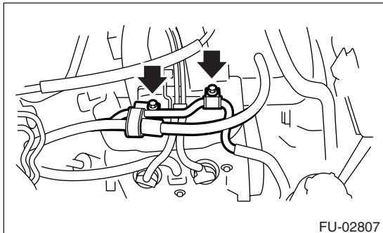
(2) Remove the installation bolt installing the power steering pump bracket.
