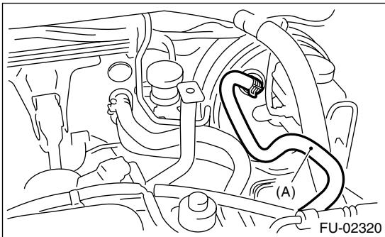
13) Connect the engine coolant hoses (A) to throttle body.
