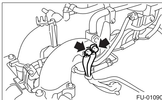
2) Remove the ignition coil & ignitor assembly. <Ref. to IG(H4SO)-7, REMOVAL, Ignition Coil and Ignitor Assembly.>
