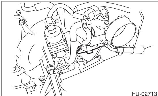
9) Connect the connector to engine coolant temperature sensor.
