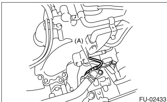
(4) Remove the reservoir tank from the bracket by pulling it upward.
