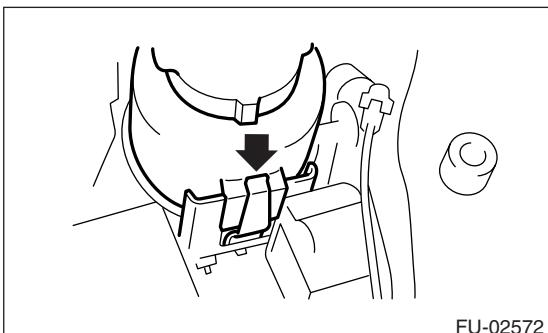
(5) Place the power steering pump on the right side wheel apron.
