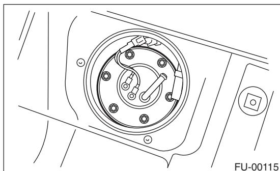
9) Remove the fuel sub level sensor.
