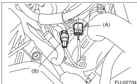
(A) Front oxygen (A/F) sensor connector
