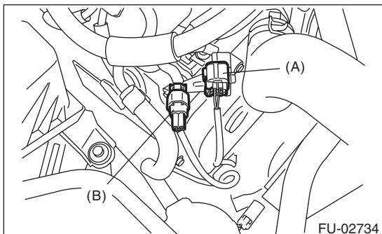
(A) Front oxygen (A/F) sensor connector
