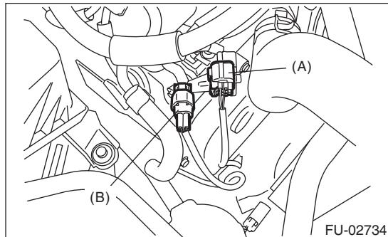
(A) Front oxygen (A/F) sensor connector
