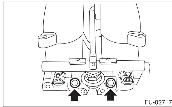
8) Remove the bolt which holds fuel injector pipe onto intake manifold.
