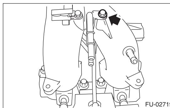
9) Remove the fuel injector while lifting up the fuel injector pipe.
