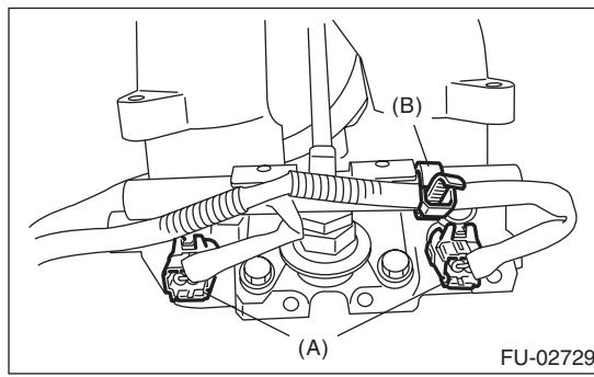
10) Remove the bolt which holds fuel injector pipe onto intake manifold.
