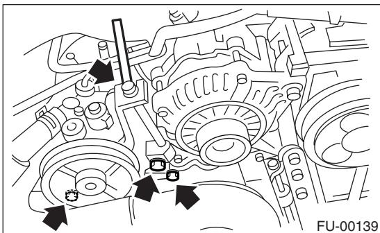
(4) Disconnect the connector from power steering pump switch (A).
