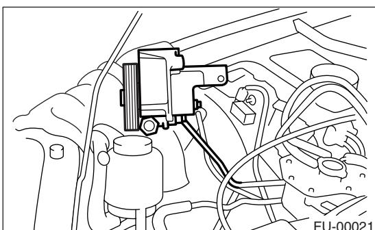
6) Remove the spark plug cords from spark plugs (#1 and #3 cylinders).
