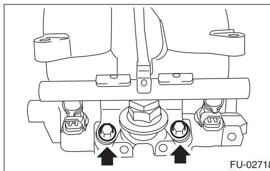
11) Remove the fuel injector while lifting up the fuel injector pipe.
