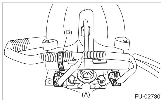
6) Disconnect the connectors (A) from fuel injector.
