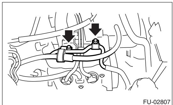
(3) Remove the bolts which install the power steering pump to the bracket.
