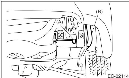
7) Remove the canister from the body.
