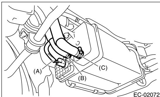
5) Disconnect the quick connector (A) from the canister.
