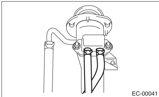
3) Remove the shut valve from the fuel filler pipe.
