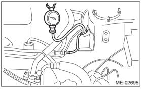
3) Connect the connector of fuel pump relay.
