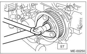
7) Remove the cam sprocket No. 1. To lock the camshaft, use the ST.
