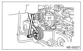
3) Remove the crank pulley.
