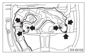
7) Remove the bolt which holds center exhaust pipe to hanger bracket.
