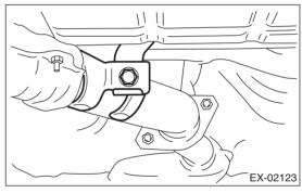
7) Tighten the nuts which hold front exhaust pipe to cylinder heads.
