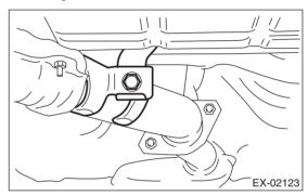
8) Remove the front and center exhaust pipe assembly from the vehicle.
