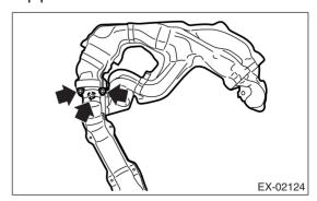
10) Remove the front oxygen (A/F) sensor and rear oxygen sensor. <Ref. to FU(H4SO)-36, REMOV-AL, Front Oxygen (A/F) Sensor.> <Ref. to FU(H4SO)-38, REMOVAL, Rear Oxygen Sensor.>
