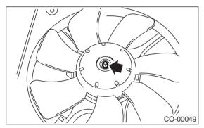
3) Remove the bolts which hold fan motor onto shroud.
