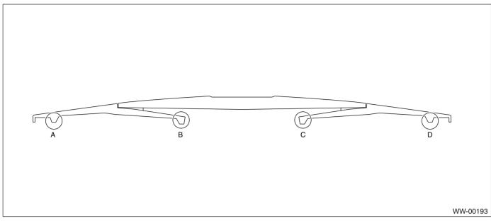
1) Insert the wiper rubber into claw (B).
