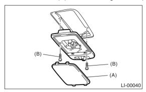
3) Disconnect the harness connector and remove the room light.
