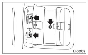
4) Disconnect the harness connectors and remove the spot map light.
