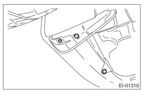
3) Turn over the mud guard, and remove one inside clip that secure the front bumper to the fender.
