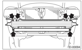
8) Remove the 8 bolts and disassemble the front bumper beam.
