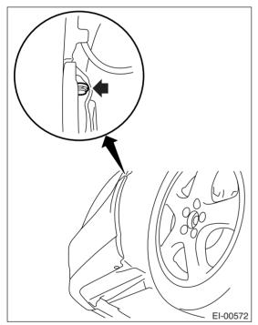
4) Turn over the mud guard and disconnect the fog light connector.
