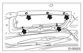
3) Remove three black clips and remove the front hood grille.
