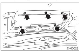
5) Hook the two hooks (A) of hood duct to the hood holes.
