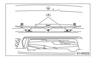
6) Install the front hood duct with the five screws and clip (A).
