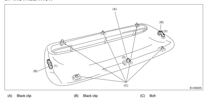
1) Replace the black clips (1) and (2) with new parts. Install the clip with arrow mark facing the front side of grille (A).
