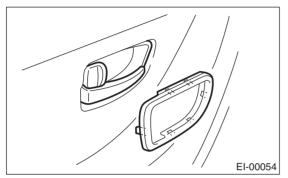
3) Remove the power window control switch. <Ref. to GW-8, REMOVAL, Power Window Control Switch.>
