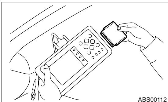
4) Connect the Subaru Select Monitor to the data link connector.
