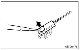
(2) Pull the connector to disconnect from the driver's airbag module assembly or the retractor assembly.
