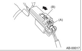
(3) With the slide lock held in the pulled position, release the lock arm (return to original position) and disconnect the connector.
