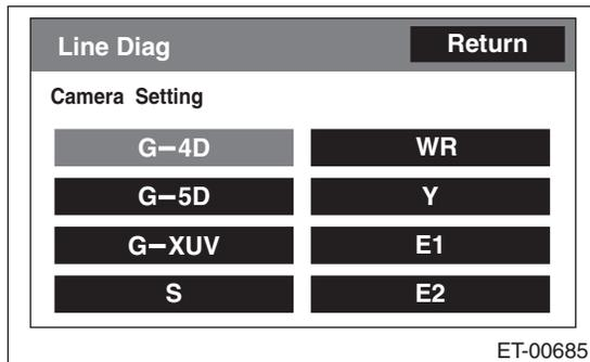
6) Shift the shift lever or the select lever to the following position to display the image of the rearview camera:
