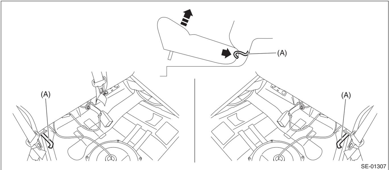
4) Remove the satellite safing sensor.
