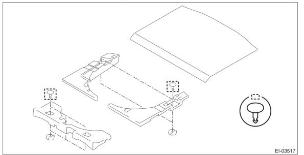
6) Remove the clips, and remove the trim panel - rear skirt.
