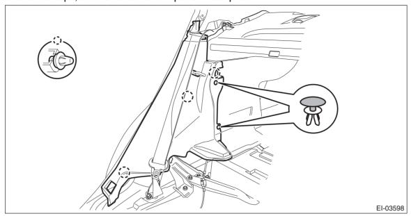
5) Remove the nuts and then remove the curtain airbag sensor. <Ref. to AB-29, SIDE AIRBAG SENSOR AND CURTAIN AIRBAG SENSOR, PROCEDURE, Airbag Connector.>
