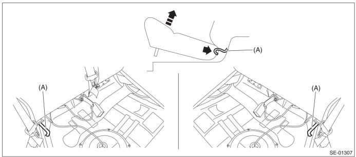
3) Release the clips and claws, and then remove the cover side sill - rear INN.
