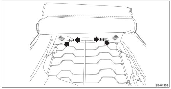
(4) Remove the pad assembly - front seat backrest and the cover COMPL - front backrest from the backrest assembly.
