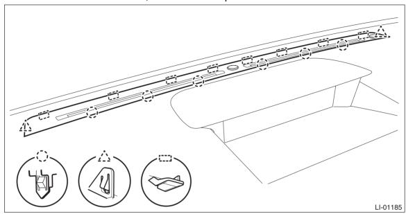
(2) Press the left and right claws to remove the sensor - sunload from the panel COMPL - instrument UPR.
