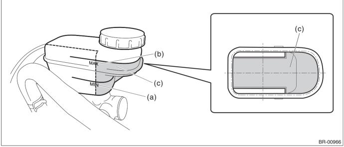
2) Check the fluid for discoloration. If the fluid is extremely discolored, replace with the new fluid.
