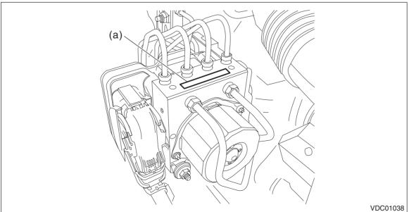
2) Check the condition of connection and settlement of connector, and correct or replace if defective.
