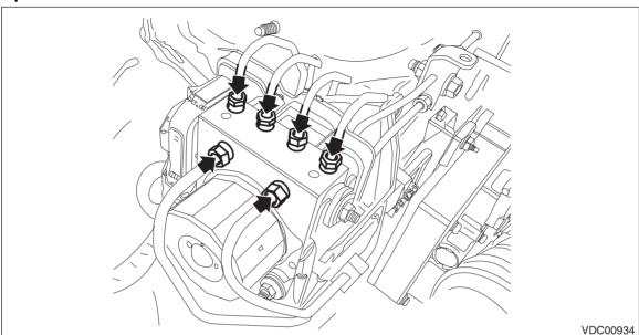
(4) Remove the nuts and remove the VDCCM&H/U from the bracket - hydraulic unit.
