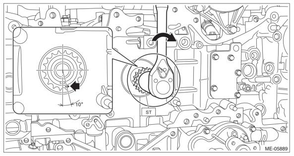
8) Using ST and by turning the intake cam sprocket LH approximately 180°, align the alignment marks of intake cam sprocket LH to the positions (zero-lift position) as shown in the figure.
