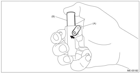
(2) With a 2.5 mm (0.98 in) dia. stopper pin or a 2.5 mm (0.98 in) (nominal) dia. hex wrench inserted into the stopper pin hole, secure the plunger.
