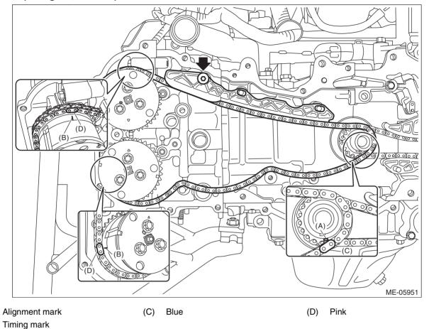
(A) (B) 6) Install the chain tensioner lever RH (A) and chain tensioner RH.
