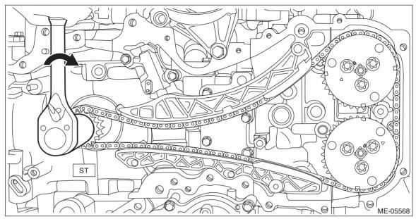
11) Install the timing chain RH. <Ref. to ME(H4DO)-122, TIMING CHAIN RH, INSTALLATION, Timing Chain Assembly.>
