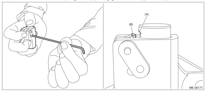
3) Using ST and by turning the crankshaft, align the alignment marks of crank sprocket, intake cam sprocket LH and exhaust cam sprocket LH to the positions as shown in the figure.
