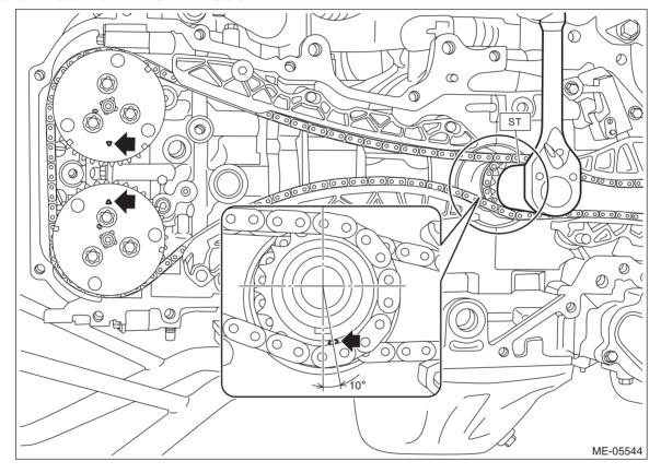
3) Push down the chain lever tensioner RH, and with a 2.5 mm (0.98 in) dia. stopper pin or a 2.5 mm (0.98 in) dia. hex wrench inserted into the stopper pin hole in the chain tensioner RH, secure the plunger (A).
