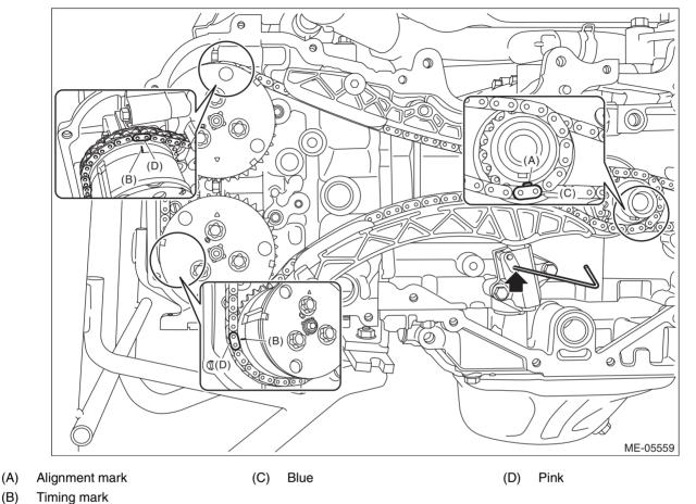
8) Using the ST, turn the crankshaft clockwise, and make sure that there are no abnormal conditions.
