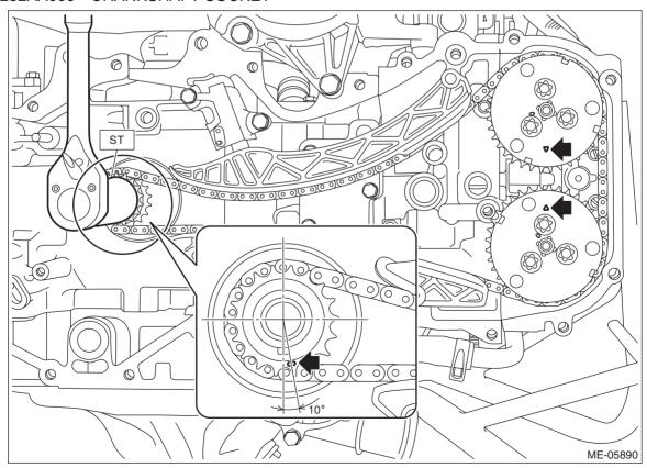
4) Align the alignment marks of intake cam sprocket RH and exhaust cam sprocket RH to the positions as shown in the figure.
