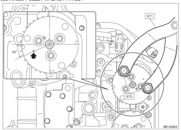
4) Using ST and by turning the crankshaft approximately 200° counterclockwise, align the alignment marks of crankshaft key to the positions as shown in the figure.
